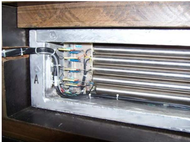
**Fig. 6.14** Shown are the position sensitive detector tubes employed on PSD at MURR. Each detector has a 1" diameter and is a 24" long stainless steel tube. The outer wall is the cathode, and the anode is a spring-tensioned nickel-chrome wire. The tube is filled with 8 bar of  $^3\text{He}$  and 4 bar of argon with 5%  $\text{CO}_2$  gas mixed in. The detection efficiency of neutrons with wave length  $1.48 \text{ \AA}$  is 70%.
