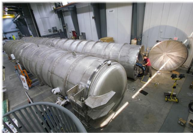
**Fig. 7.3** The cold source guide hall at the HFIR reactor at ORNL houses two SANS instruments, a 30 m and a 50 m SANS. Source: ORNL website.
