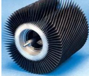
**Fig. 5.8** Shown is a velocity selector as used at the small angle neutron scattering (SANS) spectrometer Quokka at ANSTO in Australia ([www.ansto.gov.au](http://www.ansto.gov.au)). When spinning, only neutrons of a certain velocity will be able to make it past the curved blades.
