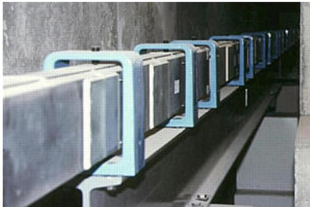
**Fig. 8.15** A neutron guide tube at the ILL reactor ([www.ill.eu](http://www.ill.eu)). Notice that, unlike a glass fiber, the tube is almost straight.
