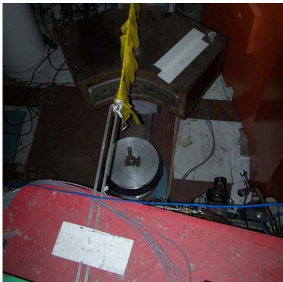
**Fig. 5.3** A straightforward diffractometer. In fact, it is one step above straightforward as this diffractometer (2XC at MURR) uses five detectors simultaneously. The openings in front of the five detectors can easily be identified in this photo, and the detectors themselves are tucked away inside of shielding material. Also visible is the sample mounted on the sample table.
