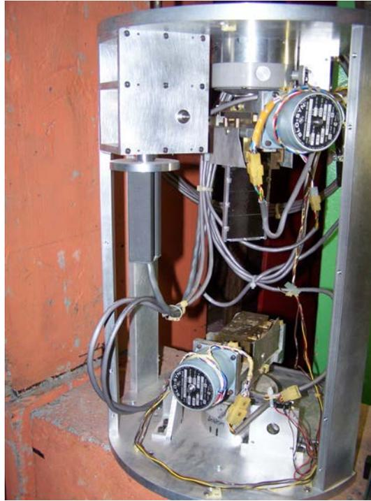
**Fig. 8.11** The monochromator of a reflectometer is flat or vertically focussing, such as the black looking stack of four graphite crystals shown here. The monochromator is oriented with the aid of several motors shown in this photo.
