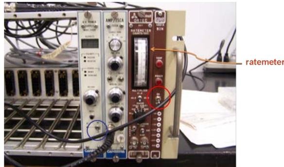
**Fig. L.1** The basic setup of the counting chain of a single detector. Note that the order of the components in the rack does not have to coincide with the logical order of the components within the counting chain.
