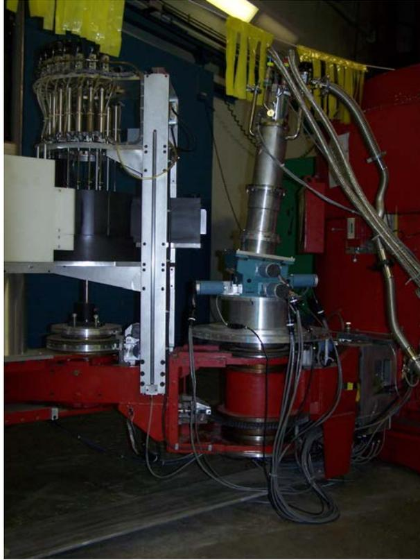
**Fig. 9.14** The tilt angles applied to the sample table under the cryostat are easily visible. This is a light weight cryostat, do not attempt these angles with a large cryostat such as a cryomagnet: it is guaranteed to break, or even lift the sample table off the floor.
