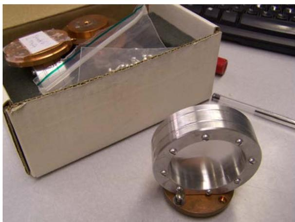
**Fig. 9.13** A strongly absorbing sample should be mounted in slab geometry, such as the one shown in this photo. This sample cell can be filled with a strongly absorbing powder; the thickness of the cell can be varied from a few tenths of a millimeter to a few millimeters. The sample cell can be housed inside a cryostat.
