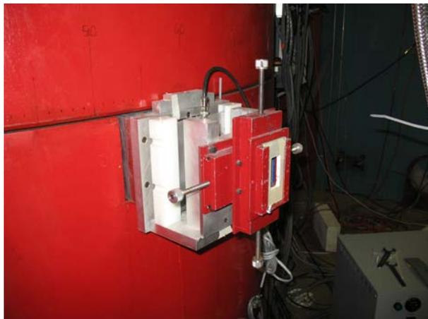
**Fig. 9.12** An example of a low-tech set of masks. The (visible) non-adjustable rectangular mask has been chosen to fairly closely match the desired beam profile. The adjustable jaws of the mask behind it (not visible) are controlled by 4 screws for adjustment (the visible screws)
