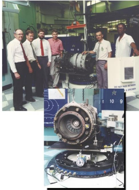
**Fig. 5.14** Tom Holden (second from left) and his team get ready to get out of the way so that they can measure strains in this turbine when it is actually spinning. This spectrometer (L3 at CINS) has since been equipped with a rig capable of applying biaxial stress. Source: [www.cins.ca](http://www.cins.ca).
