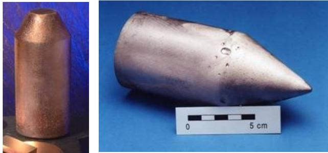
**Fig. 9.10** Images taken from the ILL website ([www.ill.eu](http://www.ill.eu)). The ILL monochromator group has succeeded in growing very large single crystals of copper (left) and a Heusler compound (right). The mosaicity of these crystals can be adjusted post-growth.
