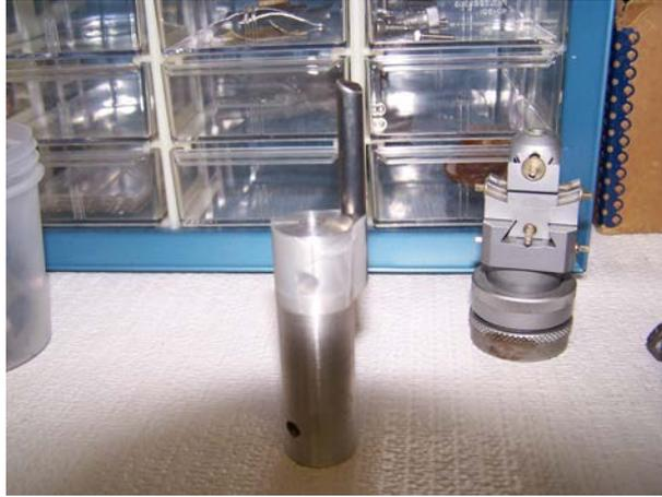
**Fig. G.2** A thin vanadium rod is placed at the center of the sample table to measure the energy resolution. Since vanadium scatters equal amounts in all directions, the mounting of the vanadium can be done by eye in an ad hoc manner as amply demonstrated in the mounting used here.
