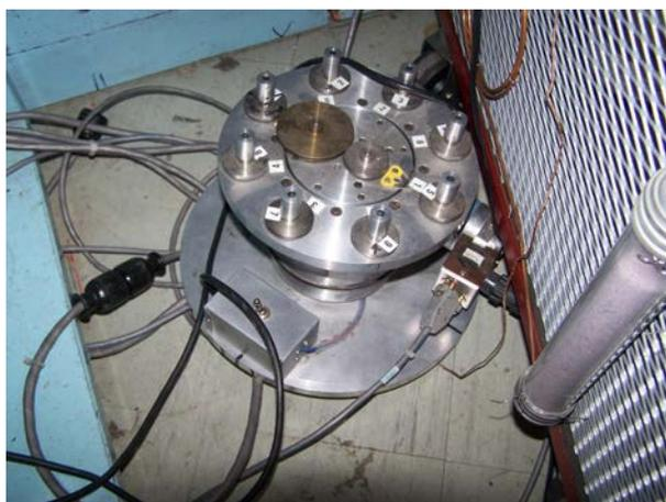
**Fig. 6.15** Typically, it does not require a lot of time to measure one powder pattern. A sample changer allows one to measure multiple patterns, and still get enough sleep.
